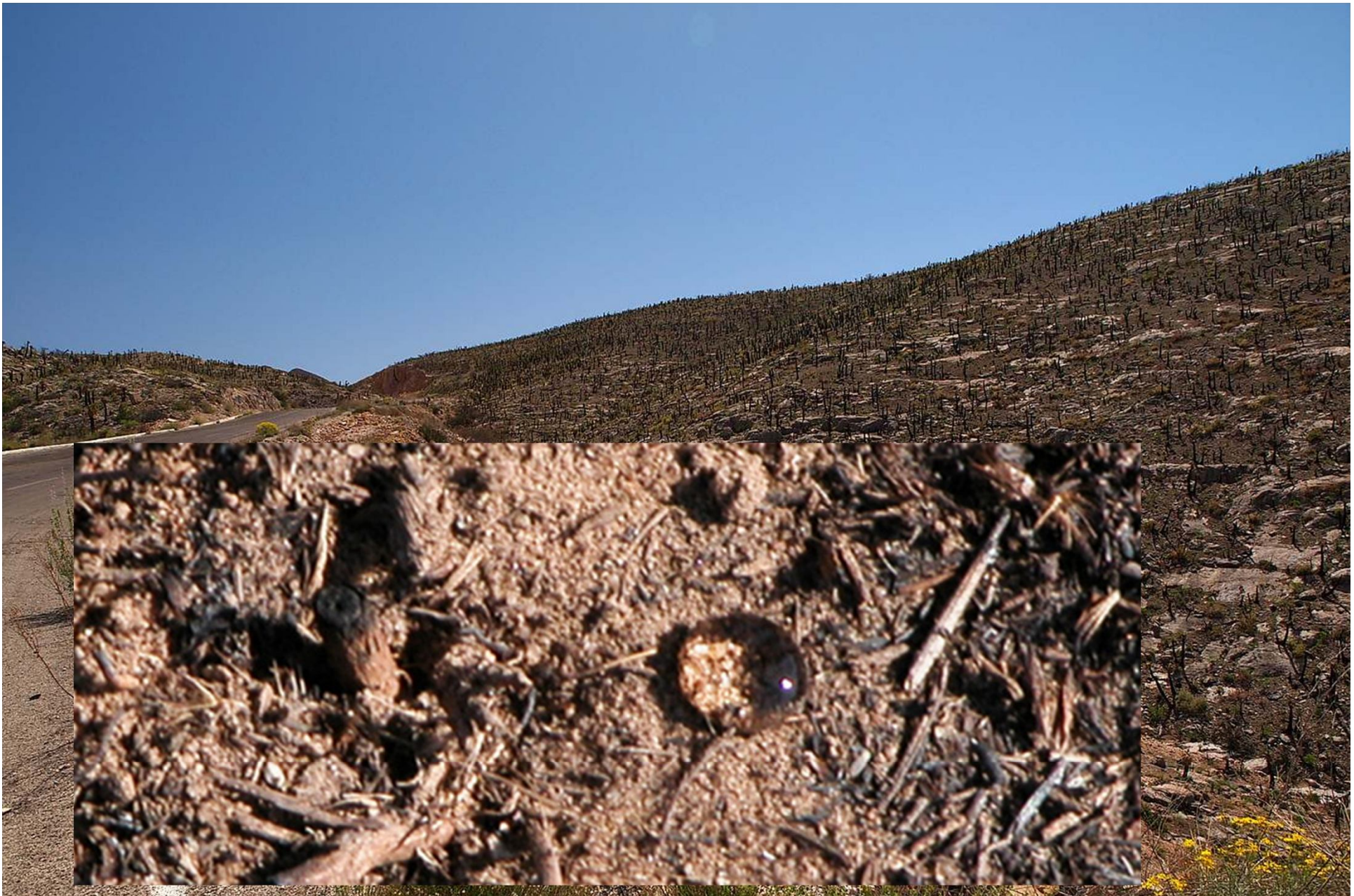
Water drop penetration test (WDPT) on the burned plot indicating a waterrepellent soil (the water drop in the picture has a diameter of approximately 1 cm).
